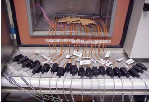
**Figure 2. Thermal Hysteresis Testing**
