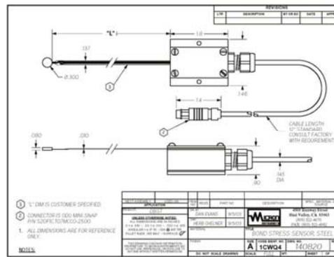
Figure 8. New DBST Sensor System
