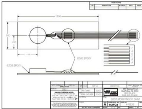
Figure 7. Sensor Bonded to Shim
