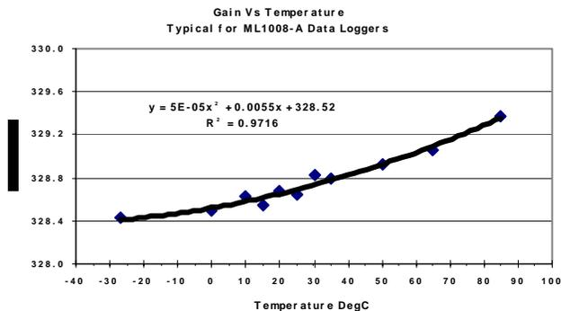
Figure 12. Effect of Temperature on Gain
