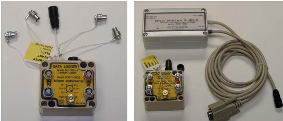
**Figure 9. ML 1008-A Logger and Interface**
