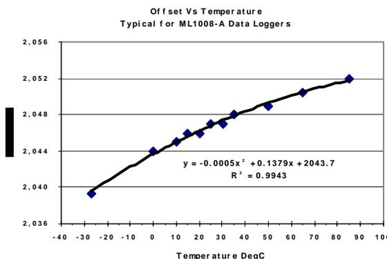
**Figure 11. Effect of Temperature on Offset**
