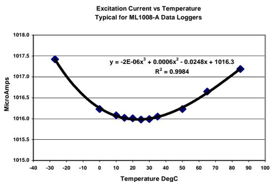
**Figure 10. Effect of Temperature on Excitation Current**
