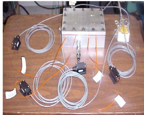
**Figure 4. Pressure Test Bomb**
